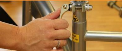
Release the hydraulic latch to allow platform adjustment. Close latch once platform is in desired position
