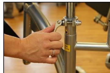
Release the hydraulic latch to allow platform adjustment. Close latch once platform is in desired position
