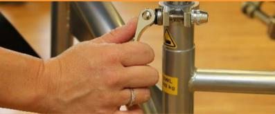
Release the hydraulic latch to allow platform adjustment. Close latch once platform is in desired position
